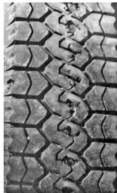
Example of Dyno Damage
