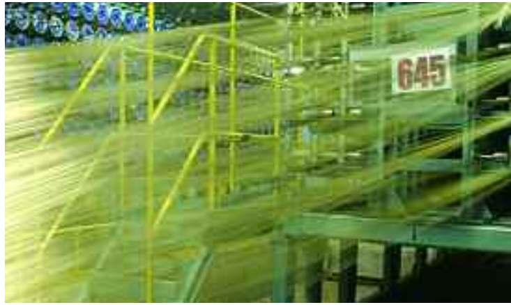
Treating steel wire with the metal cobalt – and coating it with brass formulations – helps rubber and steel to adhere to each other.
