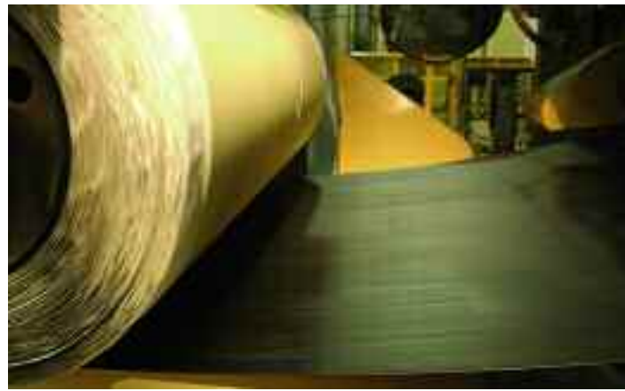
As the steel and rubber “fabric” comes out of the calender, it is wound up on rolls.
