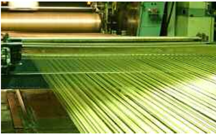
Steel cords are arranged parallel to each other and squeezed between heated rollers in a “calender” to coat the cords with rubber.
