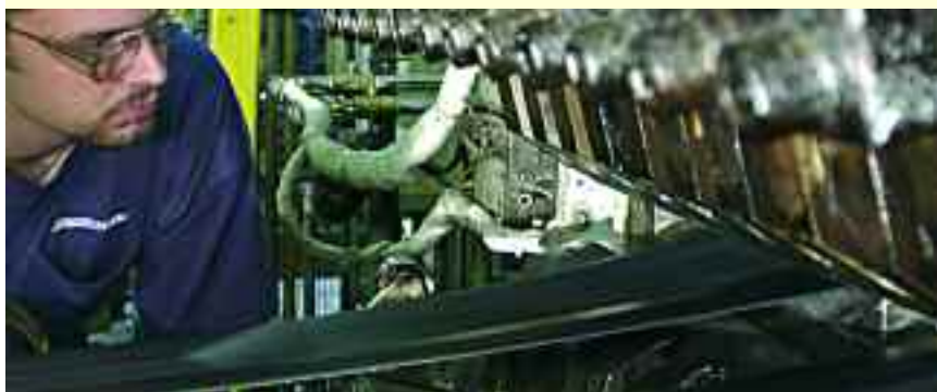
Besides calendering, the other main way tire components are made is by extrusion.
