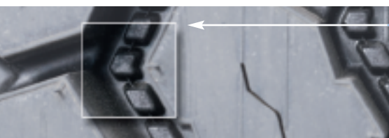
When wear bars match tread elements beside them, the tire is worn to 2/32'' .
