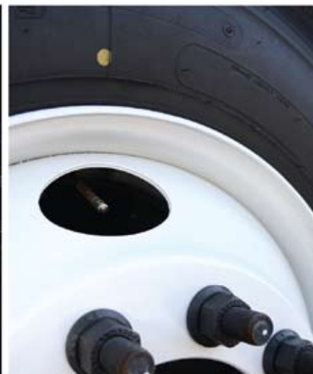
If the tire has no red dot, match the yellow dot to the valve stem.
