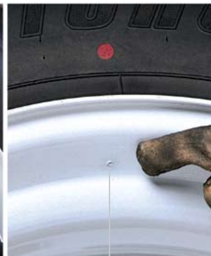
If the tire has red and yellow dots, ignore the yellow dot and match the red dot to the steel wheel low point dimple.
