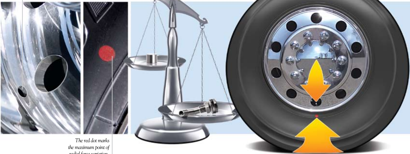
The only asymmetrical hole bored into aluminum wheels is the hole where the valve stem will be mounted.
