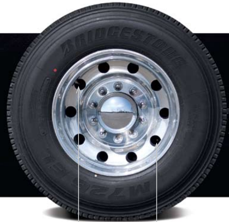
Aluminum wheels are machined, rather than forged, giving them a very uniform balance, and each hole in the wheel is matched with others opposite it to preserve that balance.
