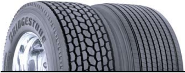
Wide base single tires, like Bridgestone Greatec drive and trailer tires, can reduce both weight and fuel costs, but require an investment in special new wheels.
