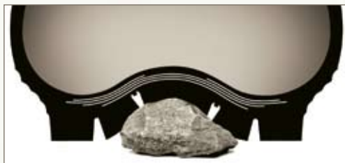
A rigid belt package cannot flex over damaging debris. And, like this refrigerator biscuit package, could tear open, exposing the casing to damaging air and water. M775’s split belt design is flexible and envelops large sharp rocks and other damaging debris.
