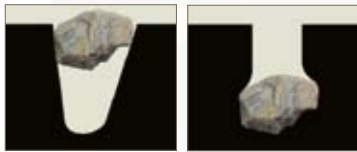
The slippery slope of the deep “V” means sharp stones can easily slide out of the groove, reducing the possibility for stone drilling.
