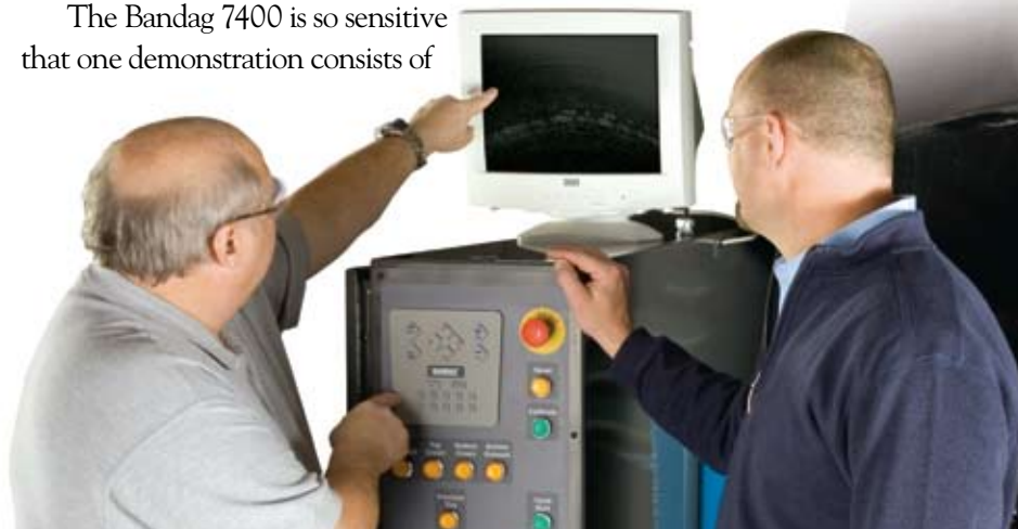
John Lindsay and Clay Timmons of Bandag discuss the interpretation of a shearography image created by the model 7400 analyzer.
